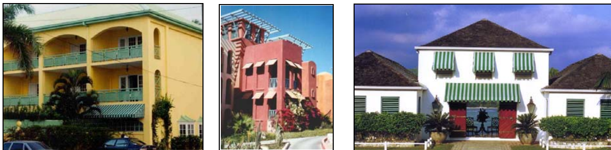
Figure 2.31 - Balcony overhangs, wooden shutters, fabric awnings and fixed louvers are all examples of effective shading devices.
